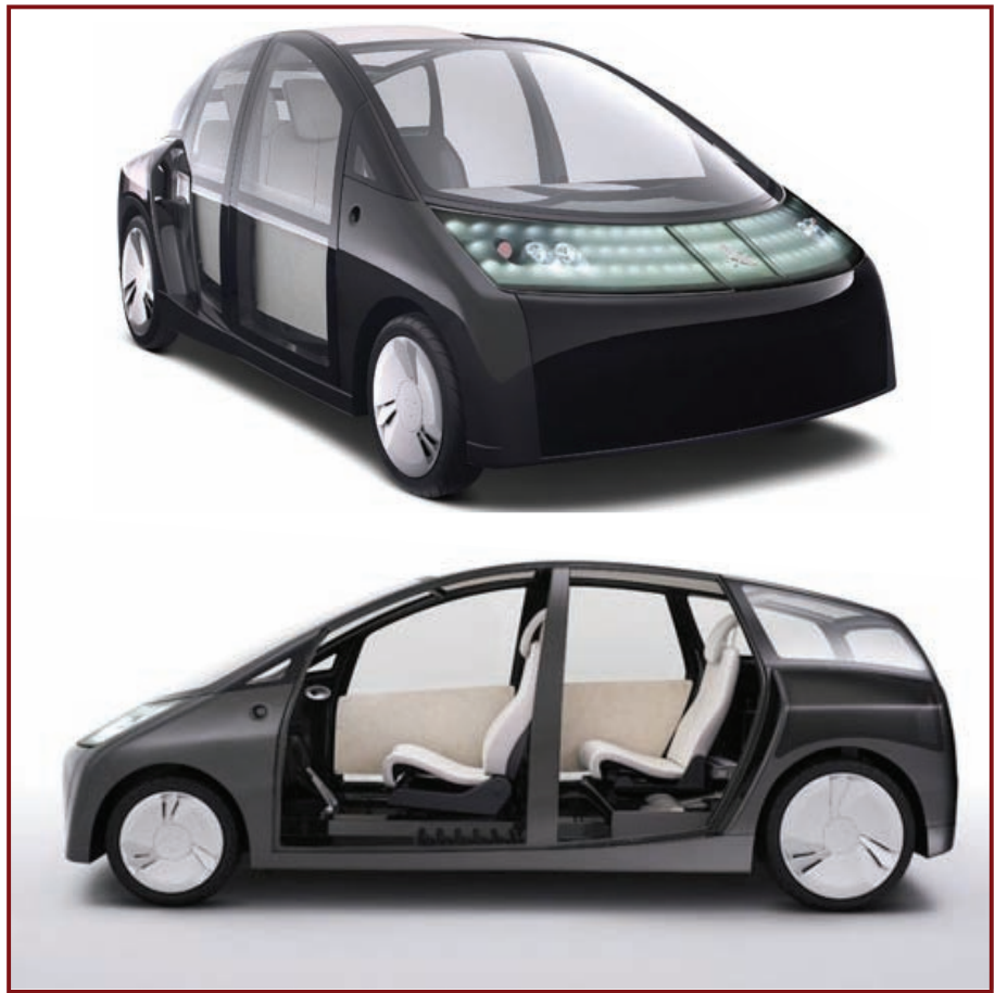
Figure 1. Toyota’s impressive 1/X carbon-fiber concept car (2007) has the interior space of a Prius midsize hybrid, but is three times lighter and twice as fuel-efficient. Its half-liter flex-fuel engine, tucked under the rear seat, is supplemented by grid electricity via 20 extra kg of batteries. A e plug-in hybrid’s remaining curb mass, 400 kg, is exactly what I’d claimed in 1991 (to much industry mirth) a good carbon-fiber four-seater could weigh.
