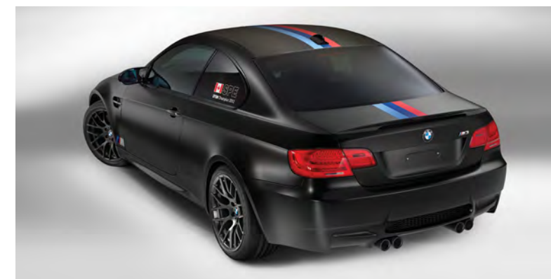
BMW's M3 (left) and Volkswagen's XL1 both incorporate carbon fiber to shave weight while maintaining strength and performance and drastically improving fuel economy.
