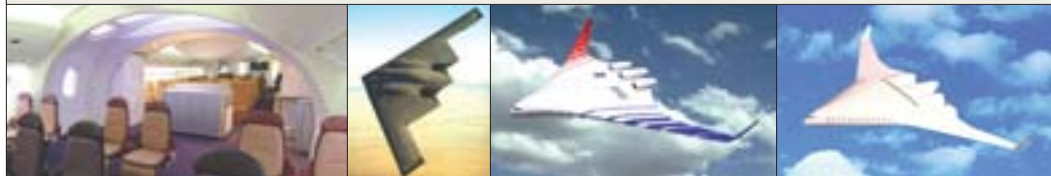
Figure 26: Next-generation airplanes. L–R: Interior vision of Boeing’s mostly-composite long-range 7E7 Dreamliner, to enter service in 2008 with 15–20% fuel saving at no greater cost; Northrop flying-wing B-2 bomber, showing how the low-signature engines of a Blended-Wing-Body design can be packed inside; artist’s conception of a civilian BWB airplane without this potentially efficiency-improving feature; 405 and an artist’s conception of a civilian BWB with ultra-efficient engine technology, embedded wing propulsion, and boundary-layer ingestion engine inlets with active flow control.
