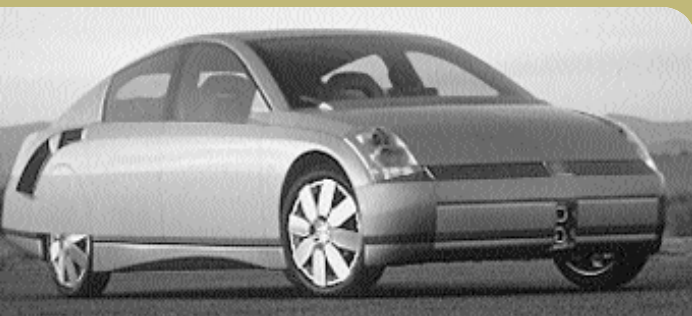
The GM Precept, possessor of one of the world's lowest aerodynamic drag coefficients.
