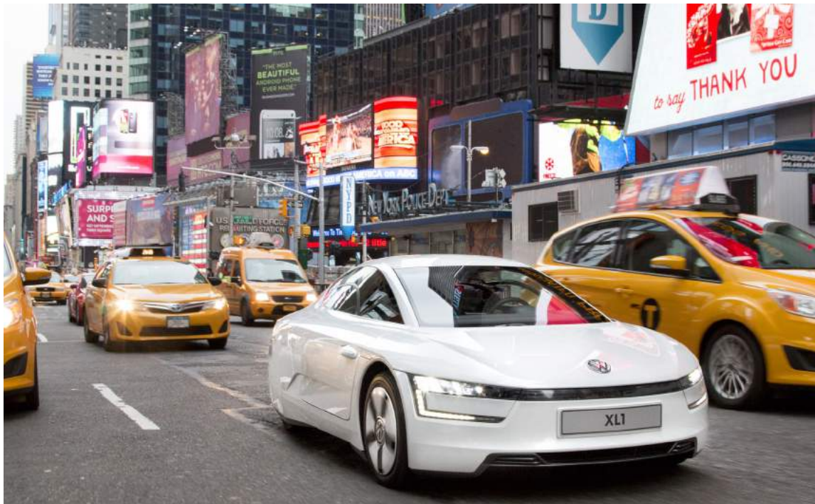
Covering the rear wheels and eliminating protruding side-view mirrors contributed to the XL1's astonishing aerodynamics.
